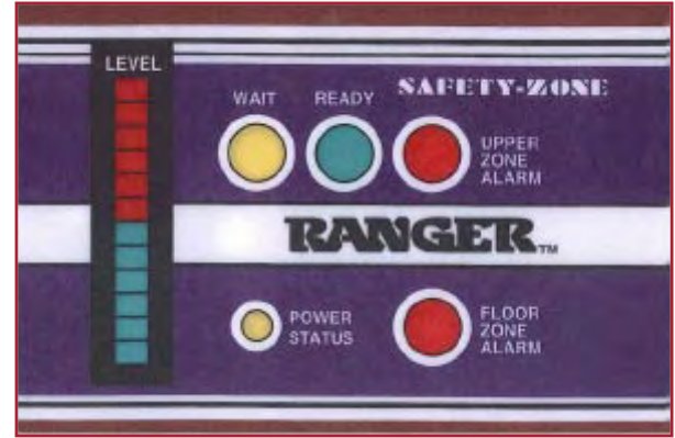
Safety-Zone Graphic Alarm Display
